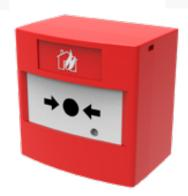
When activated, a plastic 'flag' is displayed in the window of the unit; the supplied key will reset the flag and unit. Supplied with back box.
